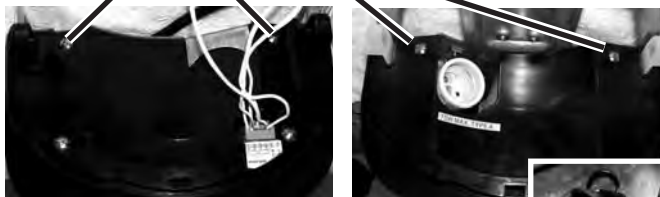
FIG. 5-2 Remove motor cover.
